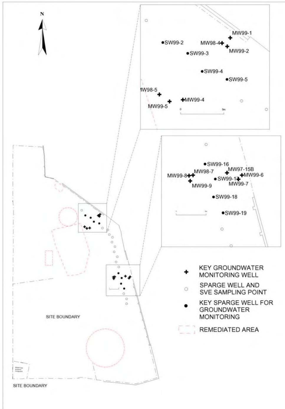
Figure 8.1: Key monitoring well and sparge well locations
