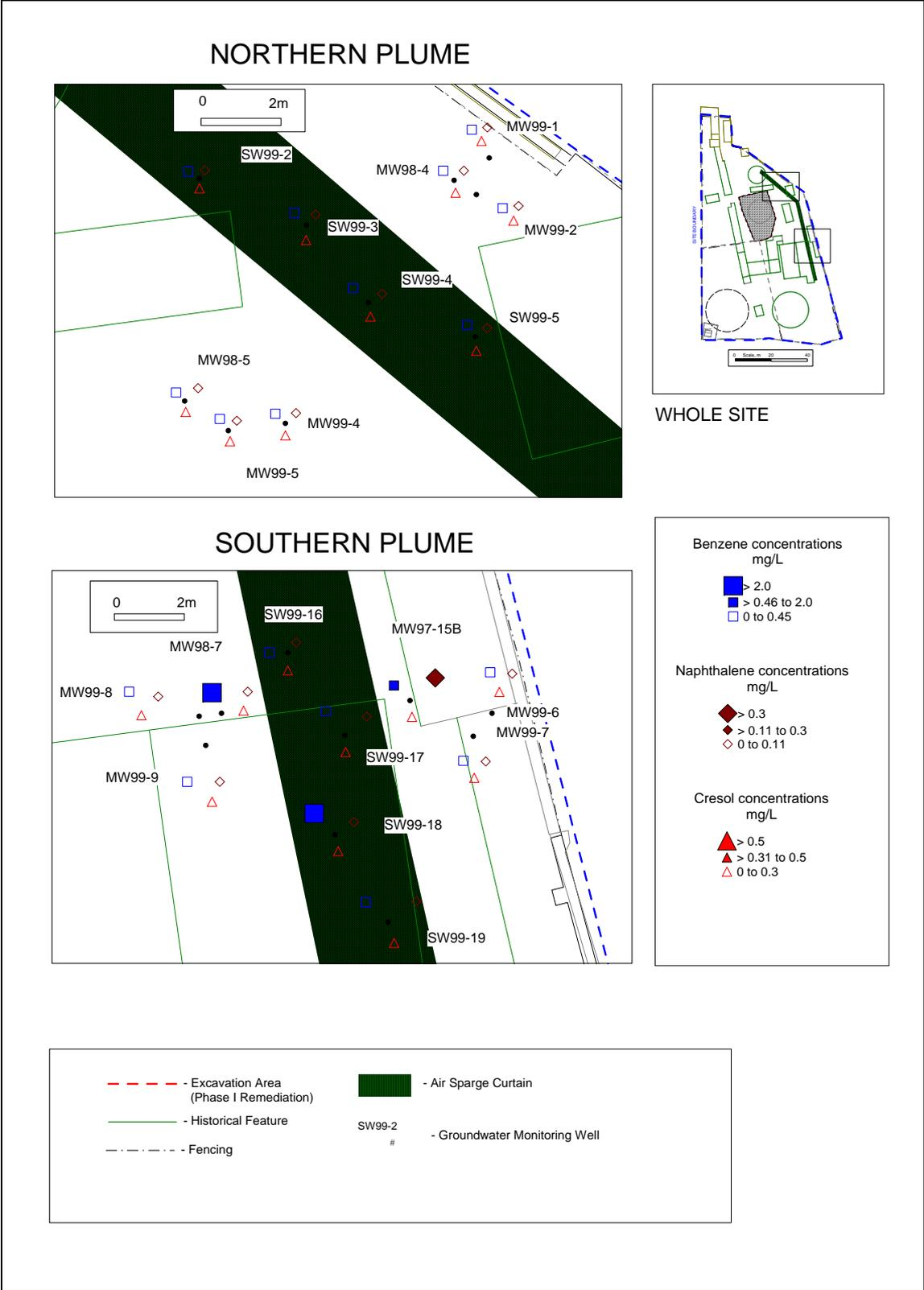
Figure 9.8: Post shutdown groundwater concentrations
