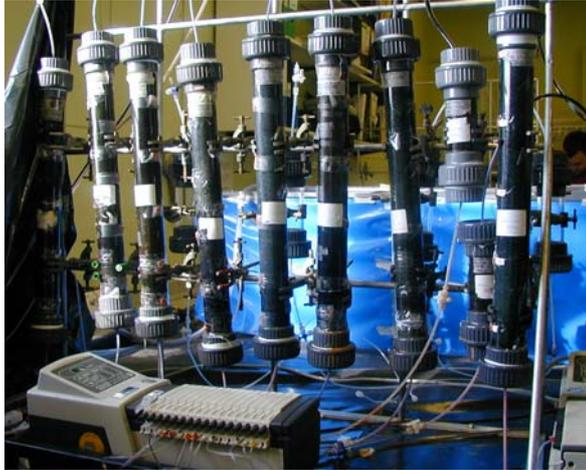
**Plate 5.1: Experimental set-up for the treatability column experiments**
