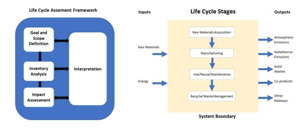
Figure 1. Overview of ISO LCA Framework (ISO 14040:2006) (left). Life Cycle Stages of an LCA (Matthews, Hendrickson et al. 2015)( right).
