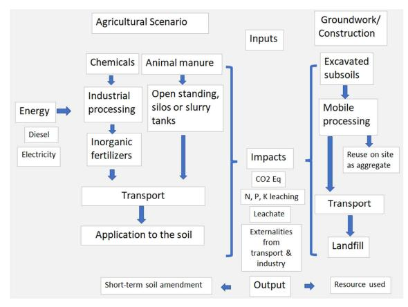
Figure 2. System Boundaries for BAU Scenarios for Agriculture and Groundworks/Construction
