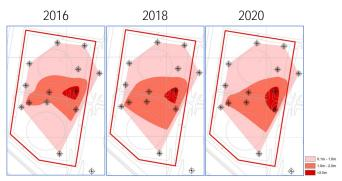
Figure 4: Median LNAPL thickness in monitoring wells (WSP).
