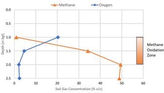
Figure 7: Typical soil gas profile, source zone (WSP).
