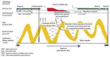
Figure 2. Schematic conceptual site model.
