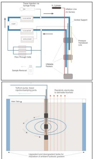
Figure 3. A conceptual model of the dipole flow and reactive tracer test (top). A schematic diagram of the dipole probe assembly (middle). A cutaway diagram of the sandbox aquifer model with the dipole located at its centre (bottom).
