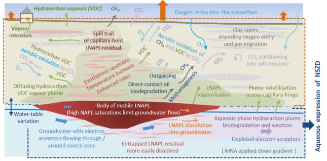
Figure 1. Conceptual site model showing processes above and below the water table generating gaseous and aqueous expressions of NSZD. The possible breakthrough of various gases ( $CH_4$ ,  $CO_2$ ) and hydrocarbon (volatile organic compound, VOC) vapours at ground surface is also shown.
