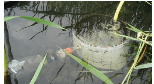
Figure 1. A typical seepage meter
