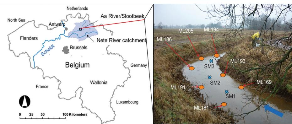
Figure 3. Slootbeek with locations for temperature measurements (ML) and seepage meter (SM) experiments
