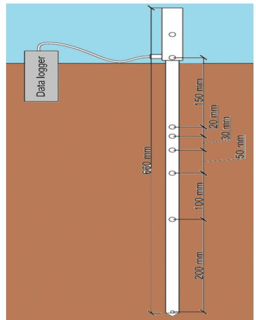
Figure 2. A multilevel temperature lance connected to a data logger. It can measure streambed temperatures at six depths as well as the streambed top.
