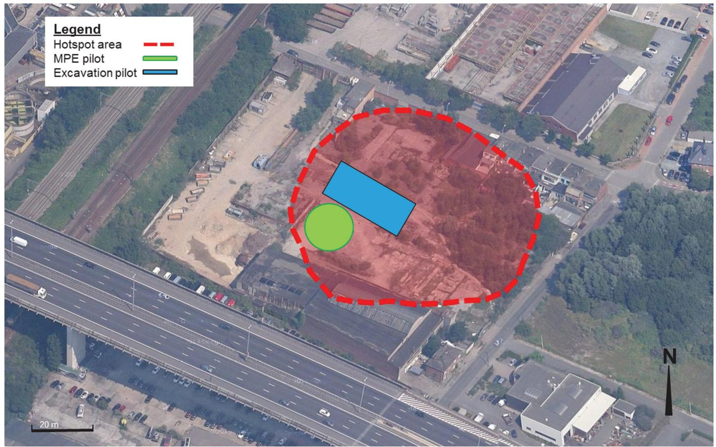
**Figure 1.** SRI Biochim site, north of Brussels. The one hectare smear zone that will be remediated on the site is outlined in red.
