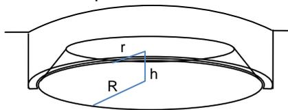
Ideally, the height of the dumpling needs to be known. This can be worked out from previous investigations, if boreholes were correctly placed.
