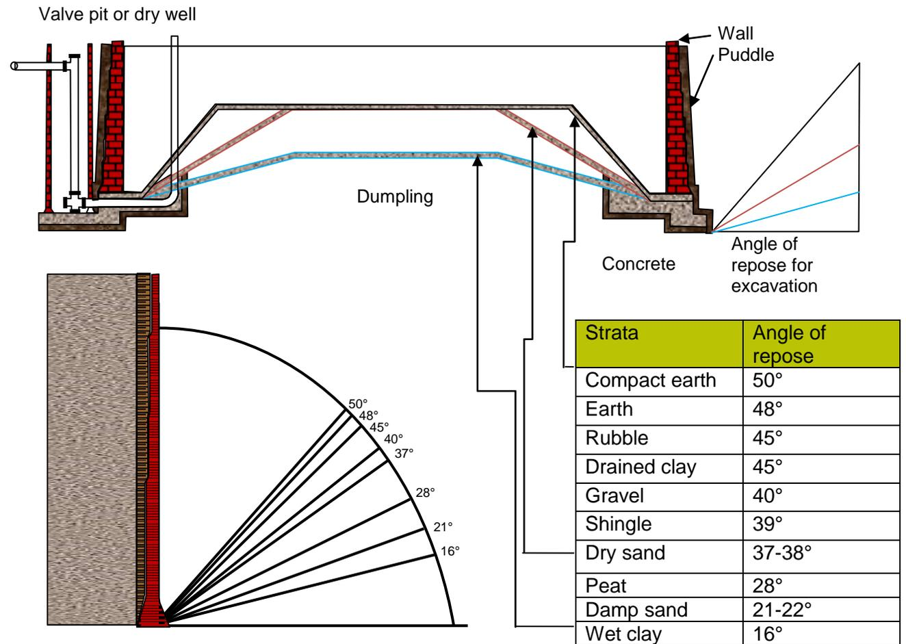
**Figure 13. The effect of ground conditions on the angle of repose when constructing an underground gasholder tank, showing angles of repose for different strata. Source: Russell Thomas.**
