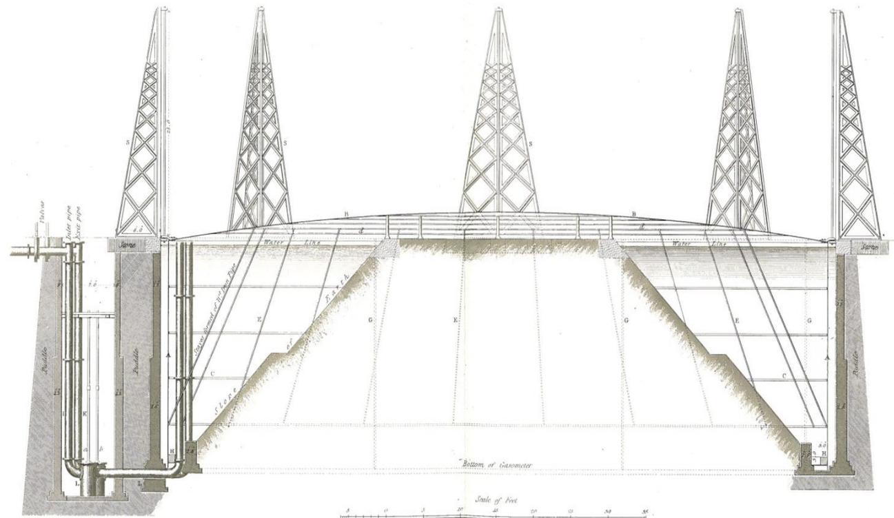
**Figure 3. Design of an early gas holder taken from 'A Practical Treatise on the Manufacture and Distribution of Coal Gas' by Samuel Clegg Junior. This simple design shows many of the features common in later gasholders. Note the basic guiding of the gasholder vessel by metal brackets with eyelets running on cylindrical metal bars; these were later replaced by guided rollers.**
