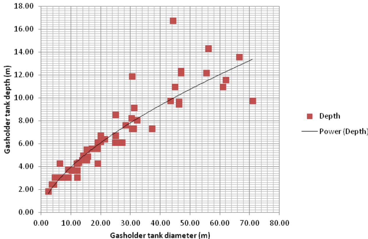
Figure 16. A plot of the gasholder tank diameter against depth for brick, stone, concrete and composite tanks. Source: Russell Thomas.
