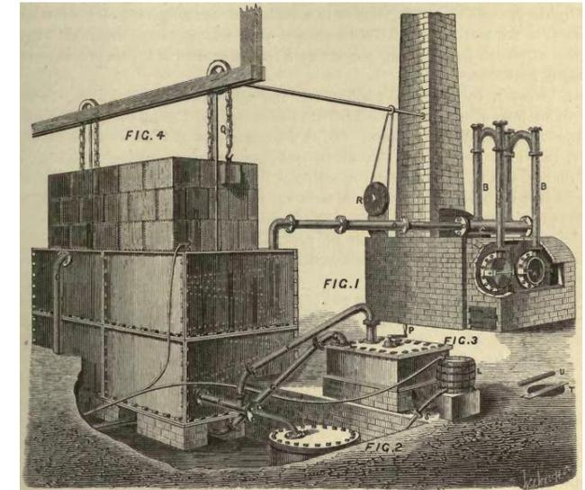
**Figure 2. The gasworks built by Clegg for Ackerman, a famous London printer, indicating the retort setting (Fig.1), tar receiver (Fig.2), lime purifier (Fig.3) and gasholder (Fig.4). From the Journal of Gas Lighting.**
