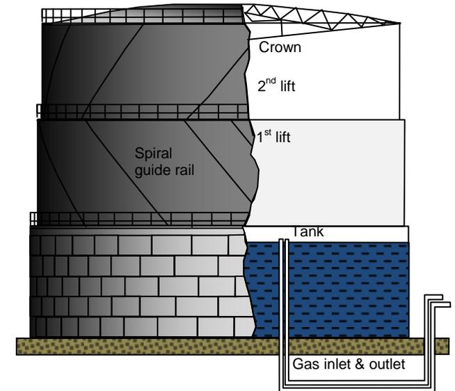
**Figure 9. Schematic of a spiral-guided gasholder with an above-ground tank, showing the internal detail and water level.**
