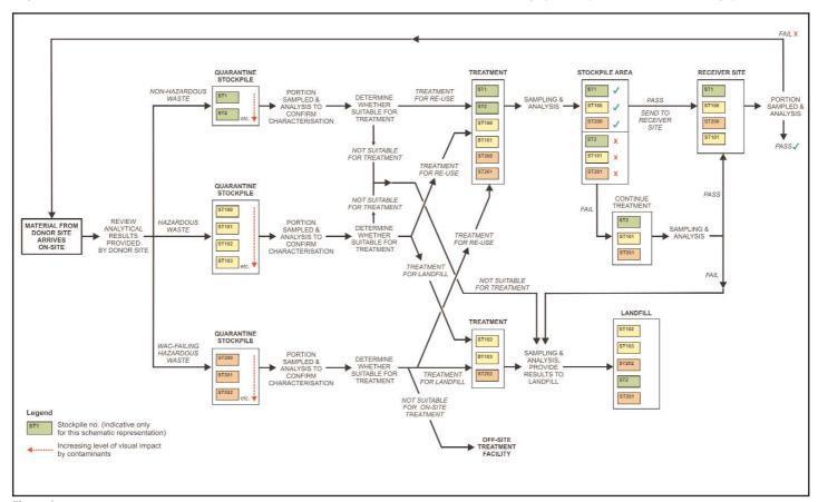
Figure 3: Schematic flowchart showing materials management.
