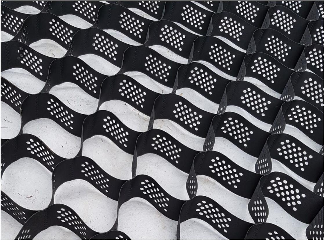
**Figure 2:** A close-up image of a geocell sheet (image courtesy of Bosky Trees)
