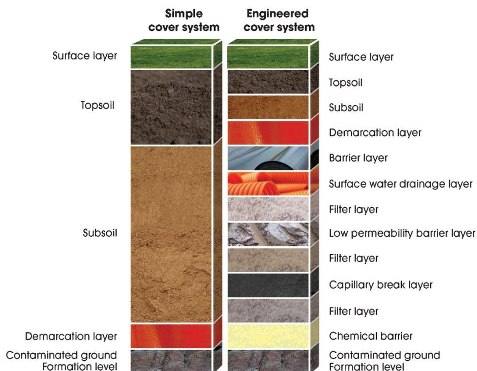
**Figure 1:** Examples of the components of a simple and engineered cover system. (Note: cover system construction is very variable and the above are examples only. Some layers e.g., a demarcation layer, may serve a dual purpose of providing a visual demarcation layer whilst also preventing intermixing)
