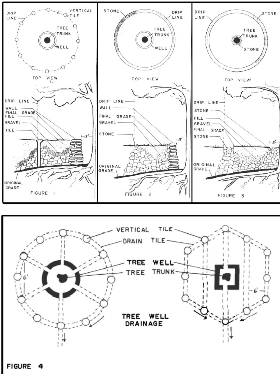
**Figure 5:** Explanatory Figures 1-4 from Collier CW, 1973, *Tree Wells, Design for Everyday Living*, Misc. Pub. 355, Cooperative Extension Service, West Virginia University. The figures show examples of different construction techniques for tree wells.
