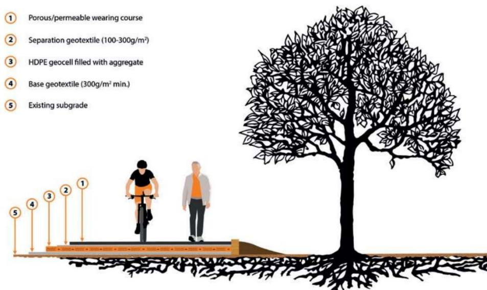
**Figure 4:** The basic approach to using cellular confinement systems near trees (image courtesy of Core LP)
