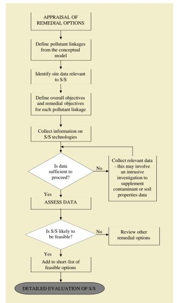
Figure 2: Flowchart to assess the feasibility of S/S at a particular site.
