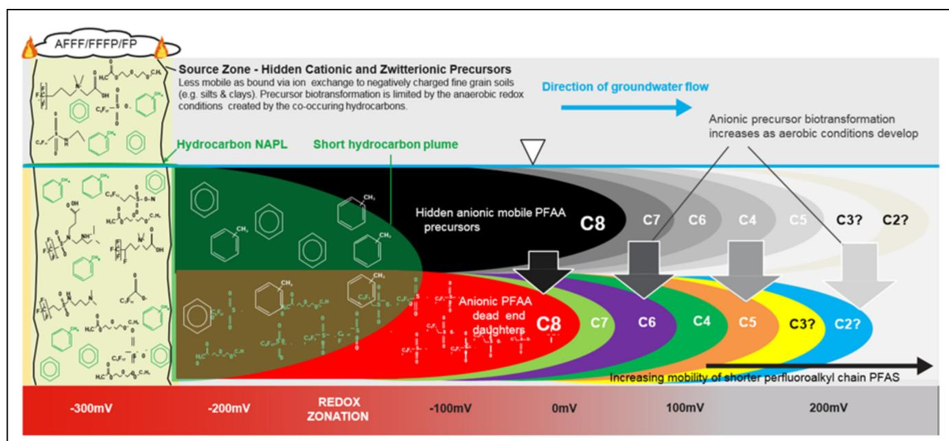
Figure 4. Conceptual site model for PFASs from a fire training area source zone.
