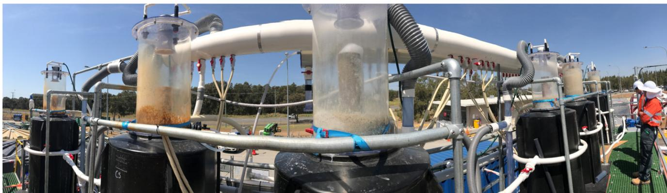
Figure 5. Ozofractionation system in action to remediate PFASs in a C6 fluorotelomer foam spill in Brisbane, Australia. Source: Ian Ross, Arcadis/EVOORA.
