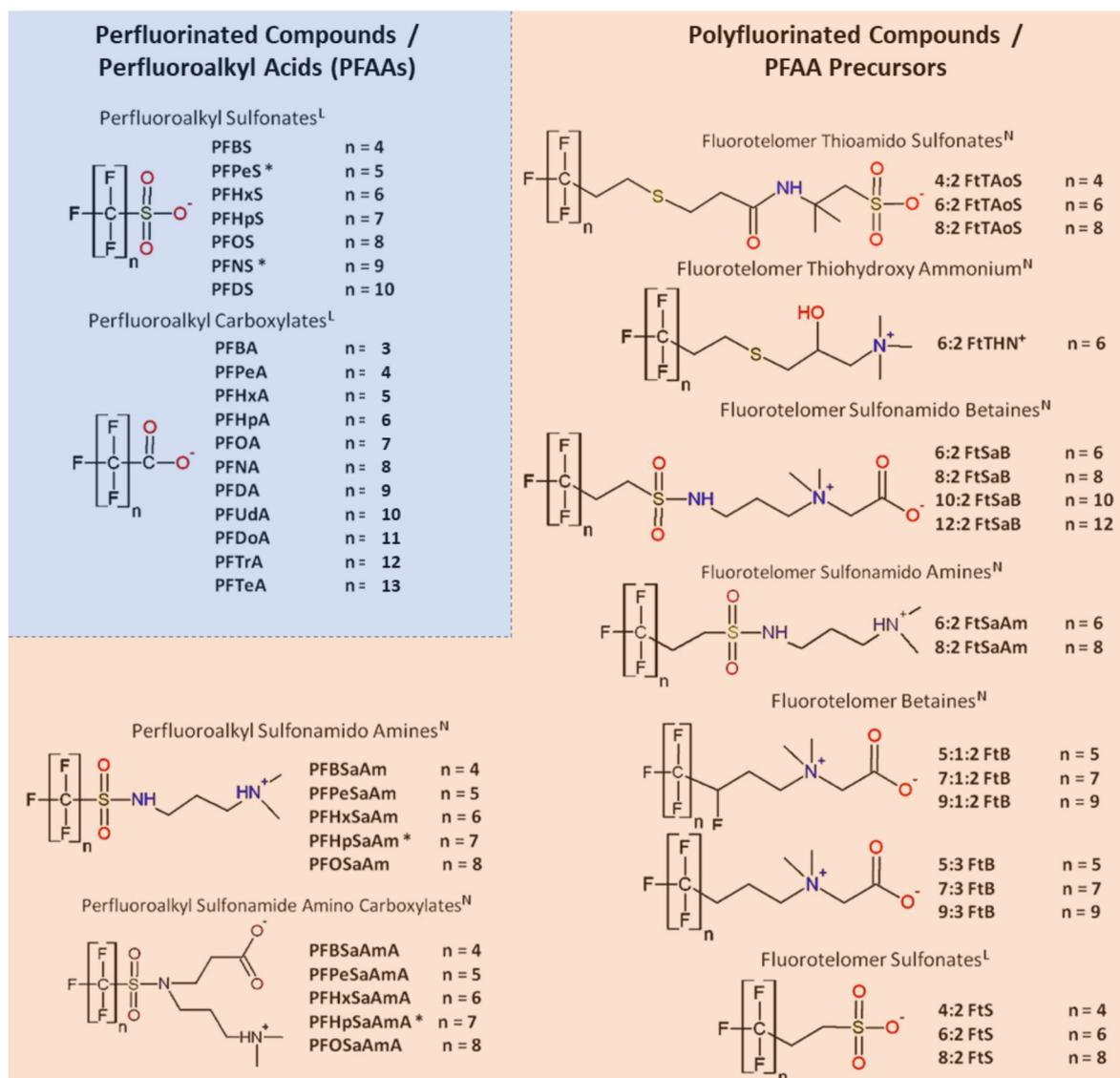
Figure 1. Examples of PFASs. Reprinted (adapted) with permission from Backe, W.J., Day, T.C., Field, J.A. 2013. Environ. Sci. Technol. 47 (10), 5226–5234. Copyright © 2013, American Chemical Society.
