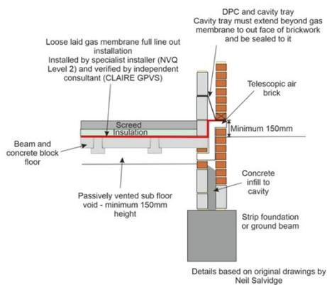
The ideal installation is to install in a "full line out" approach where the gas membrane is installed as one sheet across the floor and cavity wall. The advantages of this are:
