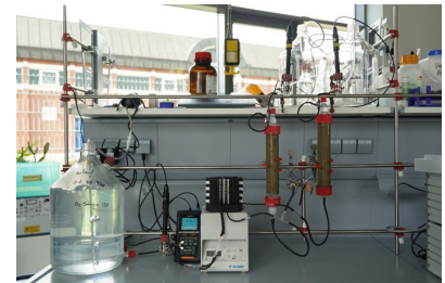
Laboratory setup to determine the soil oxygen demand of the field site.
