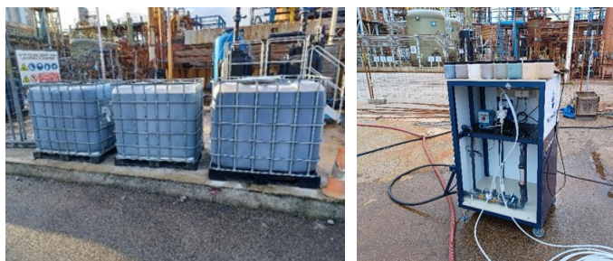
Glycerol-based substrate (left) and dosing unit (right).
