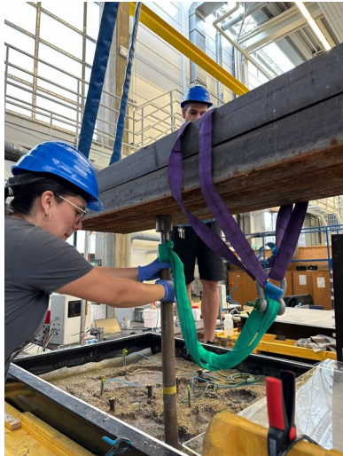
Soil extraction from ENB boxes for column experiments.
