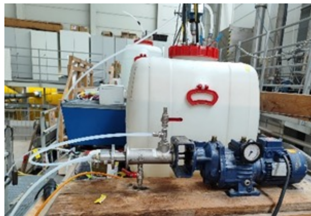
Large-scale microbial fuel cells experiment. Hydraulic set up (left) and top view of the microbial fuel cell (right)
