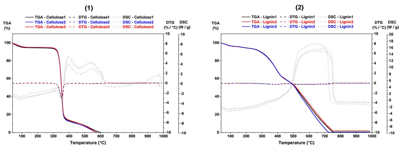
**Figure 1.** Thermogravimetric analysis (TGA) curves (*solid line*), derivative thermogravimetric (DTG) curves (*dashed line*) and differential scanning calorimetry (DSC) curves (*dotted line*) of **cellulose** (1) and **lignin** (2) (N=3).
