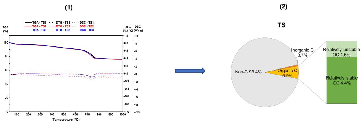
**Figure 4.** (1): Thermogravimetric analysis (TGA) curves (*solid line*), derivative thermogravimetric (DTG) curves (*dashed line*) and differential scanning calorimetry (DSC) curves (*dotted line*) of **treated sediment (TS)** (N=3); and (2) component fractions of TS: non-carbon (*grey pie slice*), organic carbon (*yellow pie slice*), inorganic carbon (*orange pie slice*); relatively unstable organic carbon (*light green bar*), and relatively stable organic carbon (*dark green bar*).
