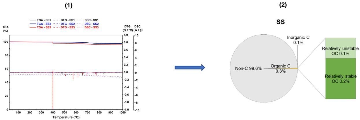
**Figure 3.** (1): Thermogravimetric analysis (TGA) curves (*solid line*), derivative thermogravimetric (DTG) curves (*dashed line*) and differential scanning calorimetry (DSC) curves (*dotted line*) of **sharp sand (SS)** (N=3); and (2) component fractions of SS: non-carbon (*grey pie slice*), organic carbon (*yellow pie slice*), inorganic carbon (*orange pie slice*); relatively unstable organic carbon (*light green bar*), and relatively stable organic carbon (*dark green bar*).
