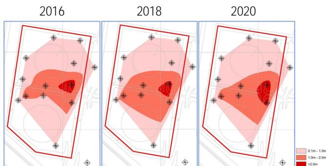
**Figure 4: Median LNAPL thickness in monitoring wells (WSP).**
