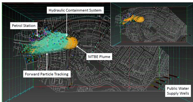
**Figure 7: Modelled hydraulic containment system capture zone and MTBE plume.**
