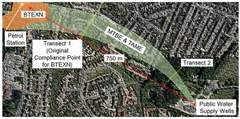
Figure 2: Schematic plan showing observed BTEXN and MTBE/ TAME plumes.
