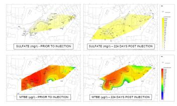
Figure 10: Sulfate and MTBE concentrations in groundwater prior to, and post, passive injection of sulfate.
