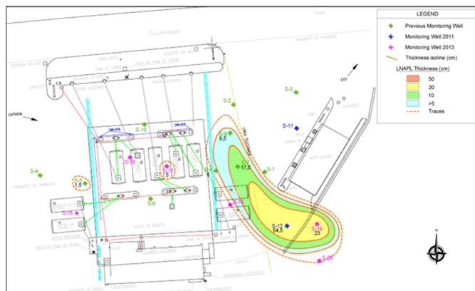
Figure 3: Thickness of the LNAPL plume, May 2014.
