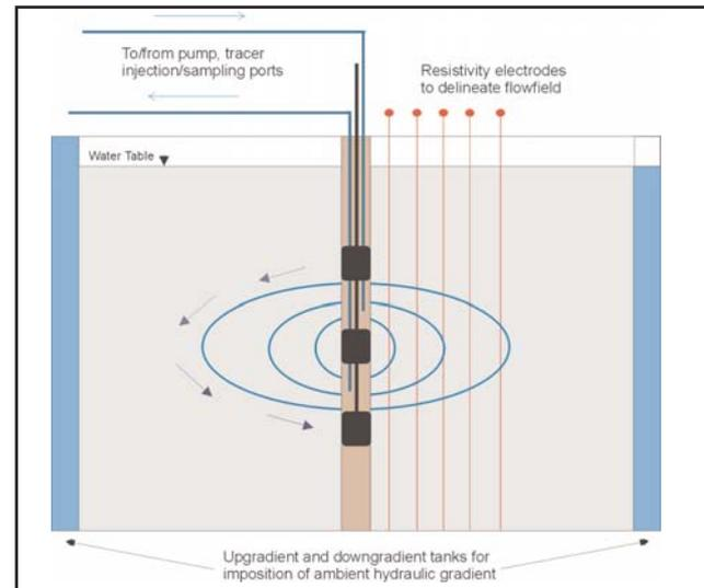
Figure 3. A conceptual model of the dipole flow and reactive tracer test (top). A schematic diagram of the dipole probe assembly (middle). A cutaway diagram of the sandbox aquifer model with the dipole located at its centre (bottom).
