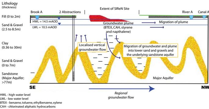
Figure 2. Schematic conceptual site model.
