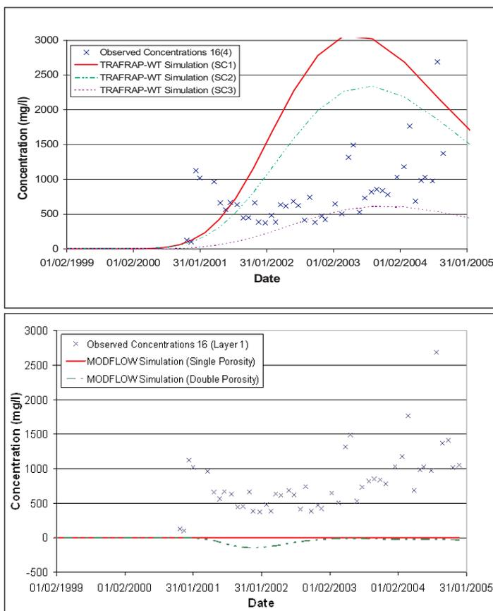
Fig.4: Performance of TRAFRAP-WT (3 scenarios) and MODFLOW/MT3DMS at Site 1 at BH16(4) for MTBE
