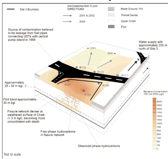
Fig. 1: Hydrogeological Conceptual Site Model for Site 3
