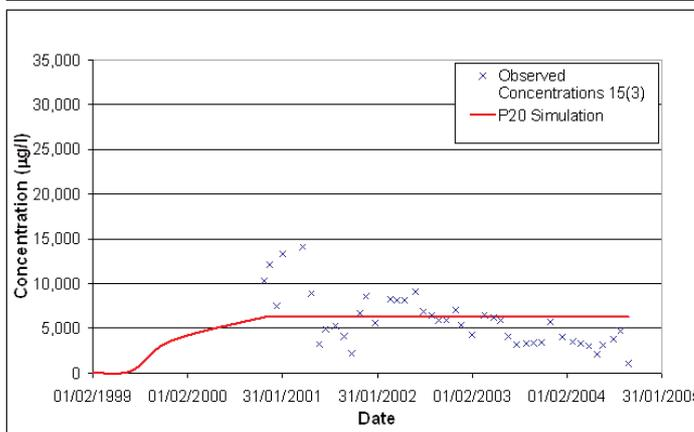
Fig.2: Calibration for benzene in BH15(3) at Site 1 using single porosity model with complex source term (top) and single porosity model with continuous source term (bottom)
