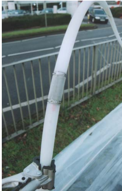
Plate 4.5: Construction of CMT multilevel sampler onsite, showing 8 cm screen section around monitoring point.
