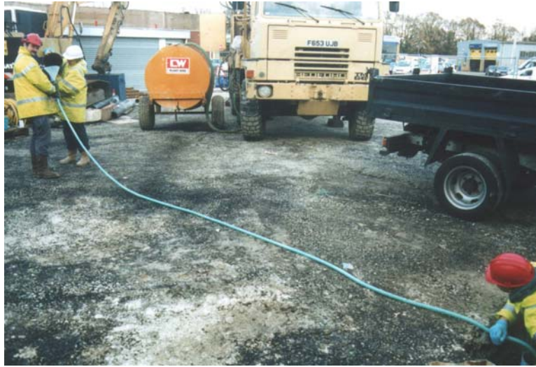
Plate 4.1: Point dilution tracer test on borehole in site source area
