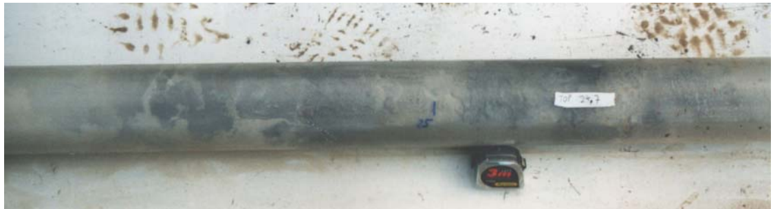
Plate 4.4: Presence of diffuse iron sulphides throughout the core from MW23, producing a grey mottled effect within the core liner
