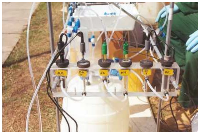
Plate 4.7: Flowcell used to obtain onsite measurements of groundwater dissolved oxygen concentration, temperature, redox (Eh), pH and electrical conductivity.
