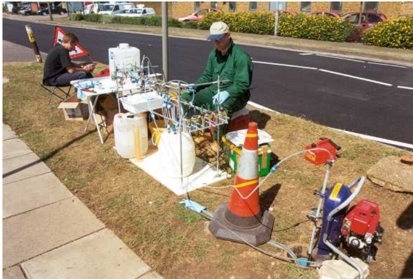
Plate 4.6: Apparatus used to collect groundwater samples, showing dedicated sampling tube from MLS monitoring well connected to the sample processing rig.
