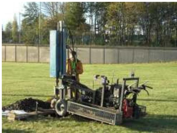
**Figure 4.55: Equipment used for core extraction**
