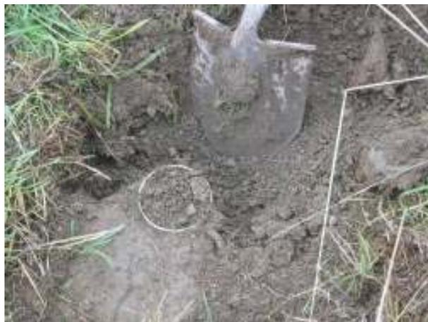
**Figure 4.26: Hand extraction of a core sample at Astra Pyrotechnics site**
