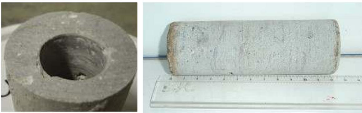
**Figure 5.4: Photograph of a fragment of core after dry cutting operation to obtain the specimens for laboratory testing**
