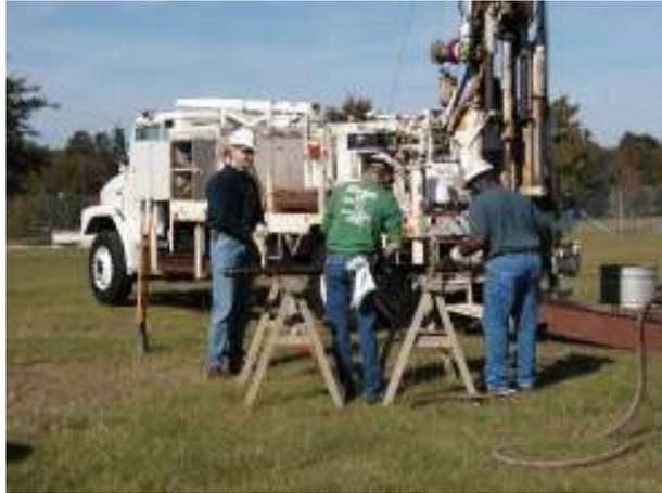
**Figure 4.55: Core barrel collection at the Columbus MGP**
