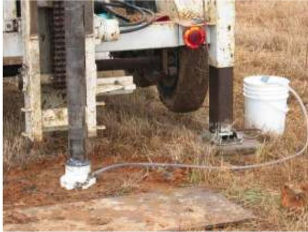
**Figure 4.19: Pressurized air system for collecting dry samples and mitigating dust generation**
