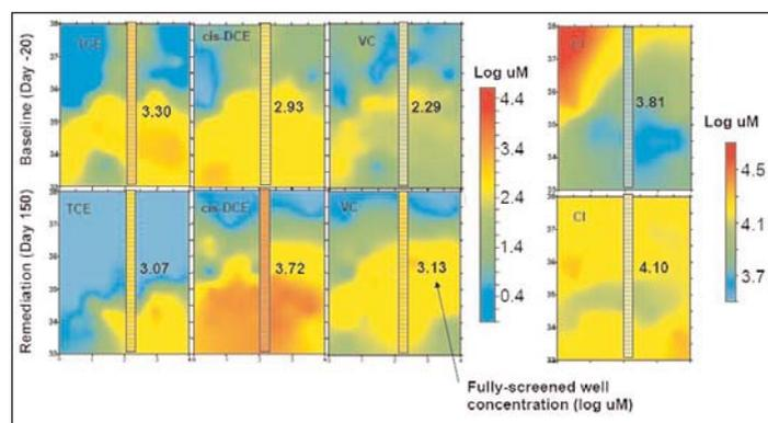
Figure 6: Comparison of plume area concentrations observed in monitoring wells and the spatial distribution of concentrations indicated by the MLS transects. Monitoring screen position is shown relative to the vertical and lateral MLS coverage. Top row is pre-remediation data; bottom row is 150 days after the start of remediation.
