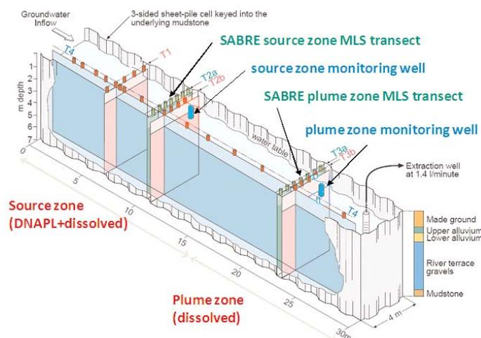
Figure 1: Schematic of the SABRE experimental test cell, showing location of conventional monitoring wells and MLS transects. Figure courtesy of the StreamTube project.
