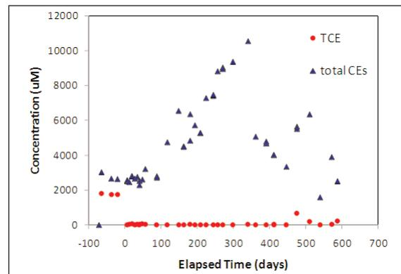
Figure 3: Temporal history of TCE and total chlorinated ethenes (TCE + cis-DCE + VC + ethene) in the source monitoring well.
