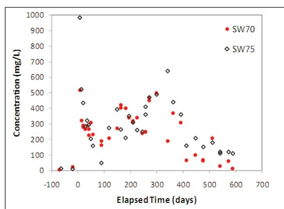
Figure 5: Total organic carbon (TOC) concentration histories in the source (red dots) and plume (open diamonds) monitoring wells. TOC is assumed to represent the amount of electron donor present.
