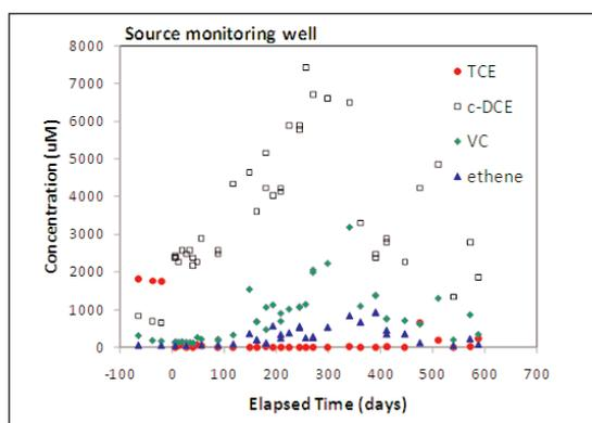
Figure 2: Temporal chlorinated ethenes and ethene concentration histories observed in the source monitoring well. Day 0 separates the pre-remediation from the post-remediation period.
