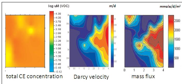
**Figure 7:** Total chlorinated ethene concentration distribution (left), Darcy velocity (middle) and total CE mass flux distribution (right) across the source fence during the remediation phase. Note that the concentration plot gives any indication of where mass is migrating. Flux maps allow monitoring of processes in space that are otherwise masked in the concentration plots.
