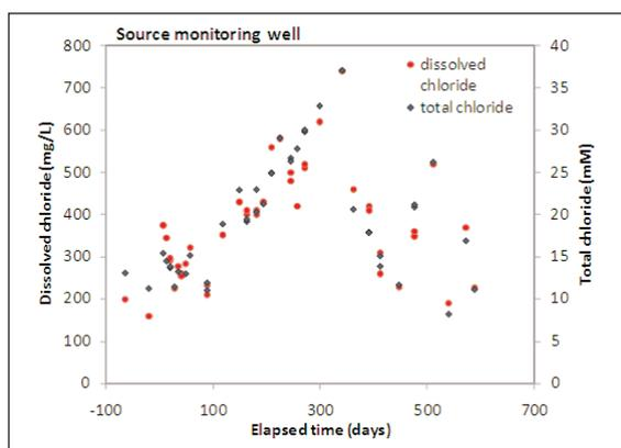
Figure 4: Total chloride and dissolved chloride observed in the source monitoring well during the experiment.
