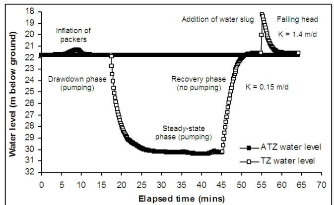
Figure 2. Example results for combined pumping and slug tests undertaken with a straddle-packer arrangement, showing response of water levels within the 2 m test zone (TZ) and above the test zone (ATZ) recorded with pressure transducers during different phases of the test (see text for discussion).
