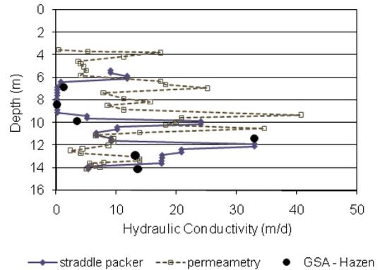
Figure 4. Comparison of K values derived from repacked permeametry and grain size analysis (GSA) of subsampled core, and straddle packer tests performed in a long screened well subsequently installed in the cored hole. Aquifer was an unconsolidated massive layered sand system.
