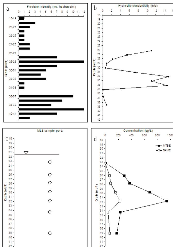
**Figure 8. Information used to design installation of MLS to monitor groundwater quality at an unleaded fuel-contaminated site on the Upper Chalk aquifer. Plots show (a) vertical fracture log; (b) aquifer hydraulic conductivity; (c) sample port location; (d) contaminant distribution obtained with completed MLS. Depth (see text) is given metres below forecourt level (mbfl).**
