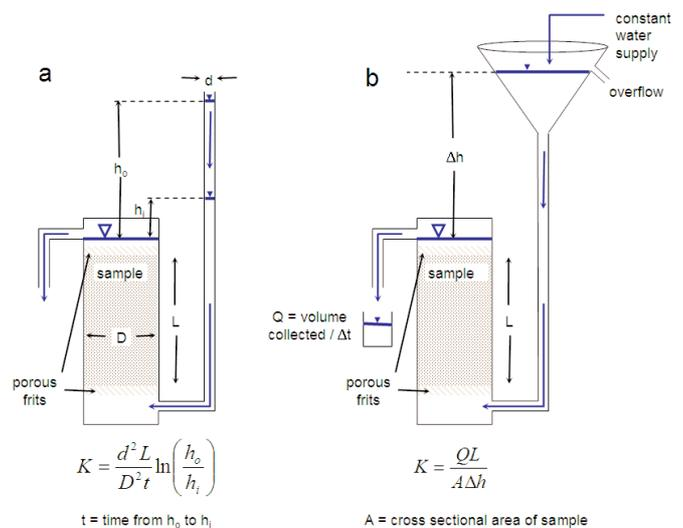
**Figure 7.** Schematic of falling head (a) and constant head (b) permeameter setups
