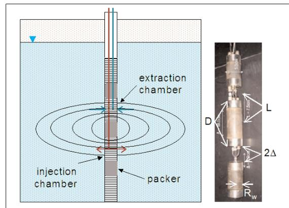
Figure 5. Schematic of dipole assembly in well and resulting idealised flowfield. Design and operational parameters are D (central packer length), L (half dipole length),  $2\Delta$  (chamber length), Q (pump rate). Dipole is constructed to fit a given  $R_w$  - well radius.
