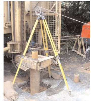
Fig.3: Set-up for downhole geophysical logging at the wellhead.
