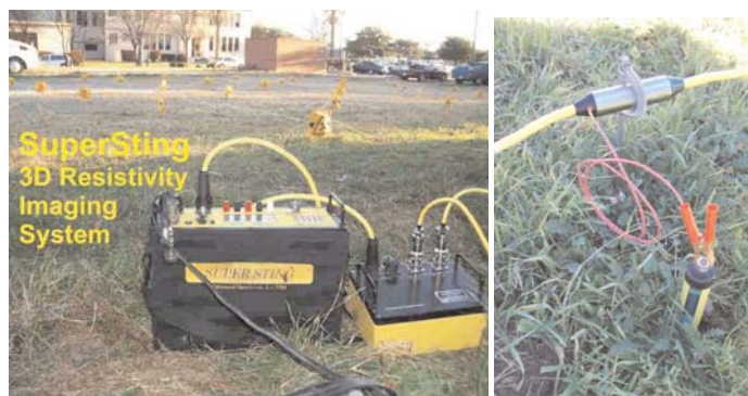
Fig.1: (left) 2-D array deployment of surface resistivity probes for 3-D tomography; (right) photo of probe tied into connecting wire of array.
