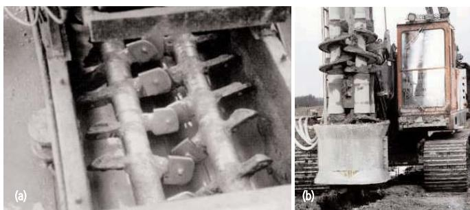
Fig 1. Examples of equipment used in the implementation of S/S: (a) a pugmill used for *ex situ* soil mixing and (b) a soil mixing auger for *in situ* mixing.
