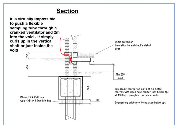
Figure 2. Incorrect approach to monitoring.
