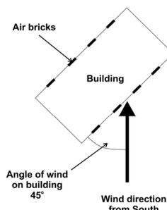
The height of the building is 5 m (the building height dictates the pressure on the wall and air bricks).
