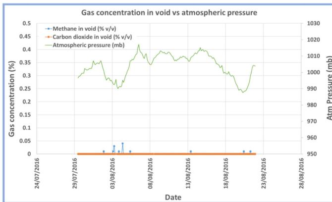
Figure 8. Gas concentrations and atmospheric pressure
