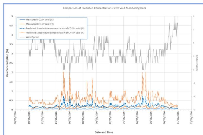
Figure 4. Comparison of predicted concentrations with void monitoring data.
