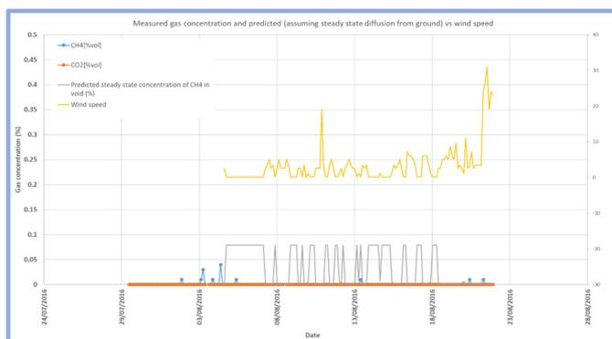
Figure 9. Measured and predicted gas concentration in void vs wind speed
