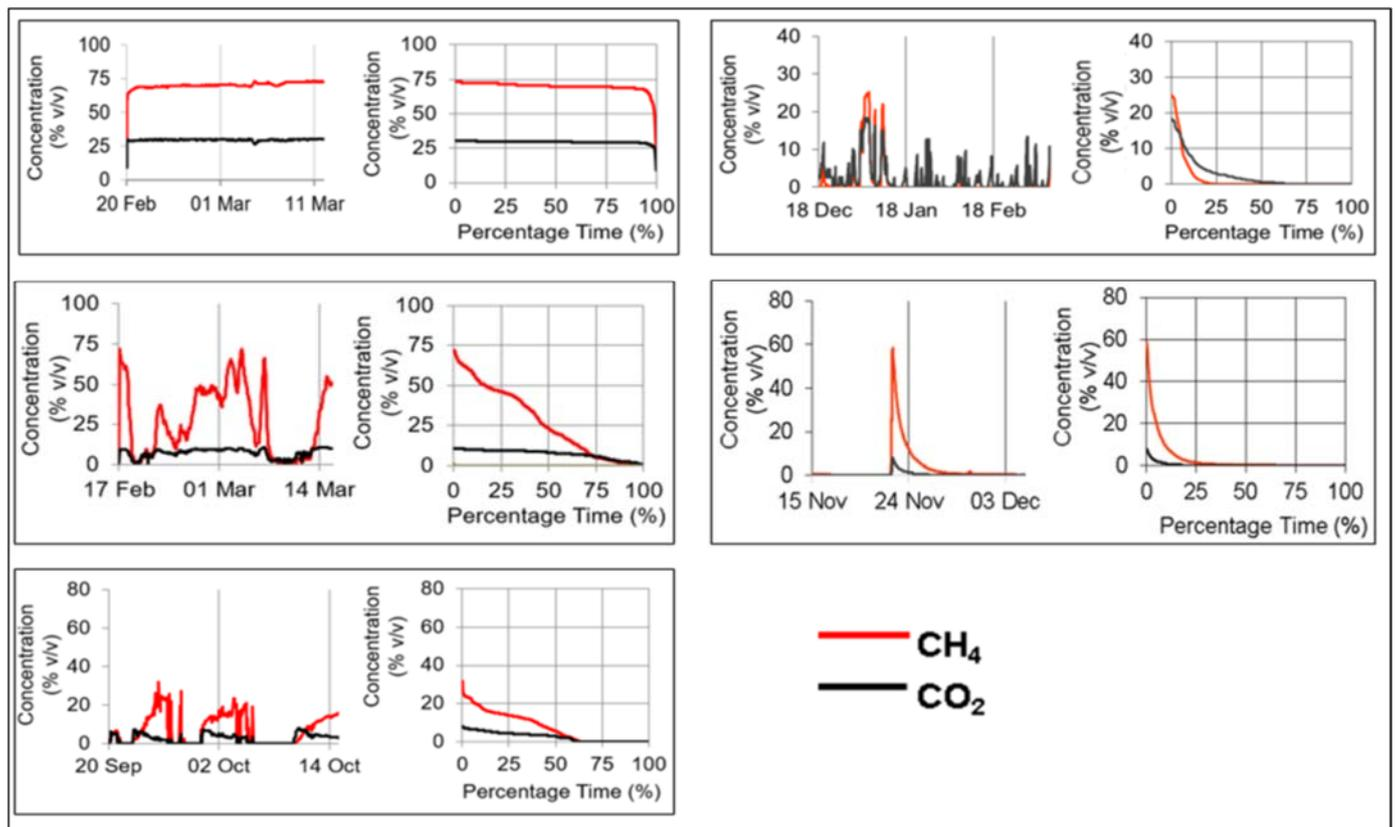
Figure 12: Families of methane (CH<sub>4</sub>) and carbon dioxide (CO<sub>2</sub>) concentration duration curves characterising position on the migration pathway from near source (top left) to extremity (middle right).
