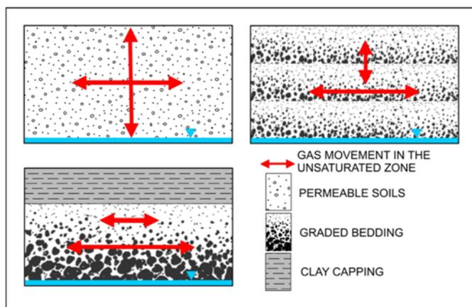
**Figure 2. Permeability anisotropy. Top left, poorly graded bedding; Top right, normally graded bedding; Bottom left, capped graded bedding.**
