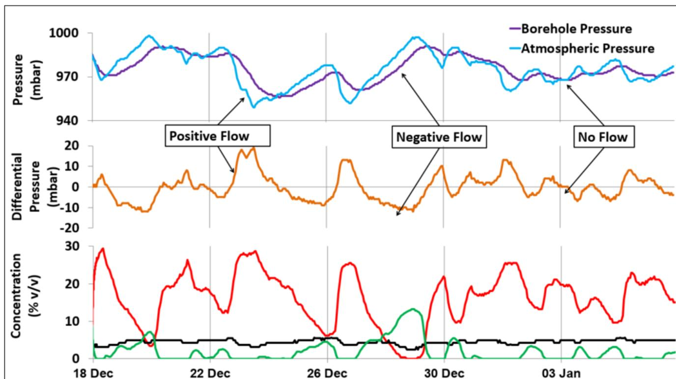
Figure 6. Relationship of differential pressure to gas concentrations.
