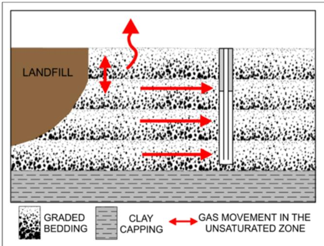
Figure 3. Horizontal permeability dominating monitoring well response.
