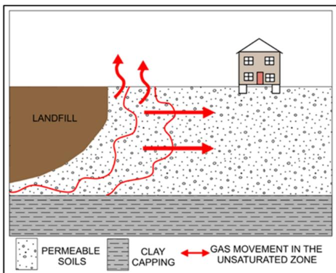
Figure 11. A ground-gas migration plume within a pathway with a source and a leading edge(s).
