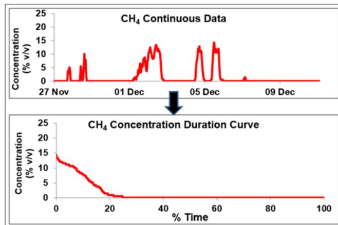
Figure 5. Conversion of time series data into a concentration duration curve.
