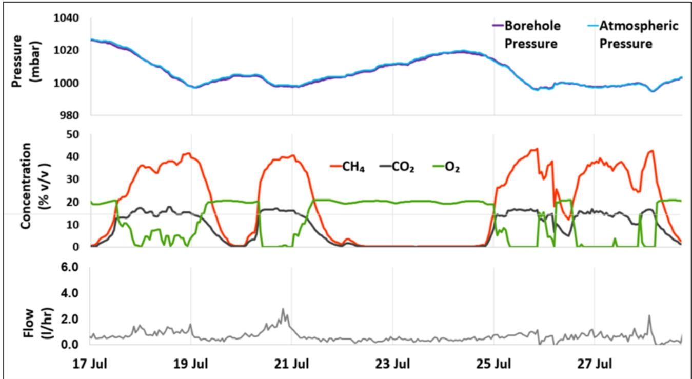
Figure 7. Relationship between pressure, continuous concentration and continuous flow.
