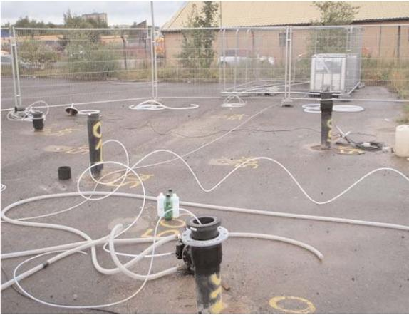
Figure 3: Groundwater re-circulation trial with abstraction well in foreground
