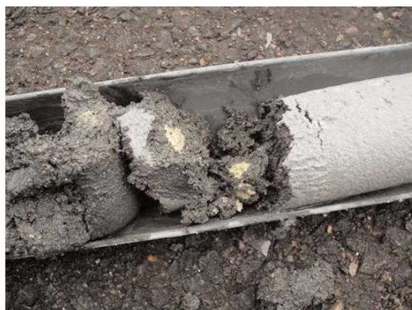
Figure 13: Presence of un-reacted Cr(VI) in soil sample on completion of soil mixing trial
