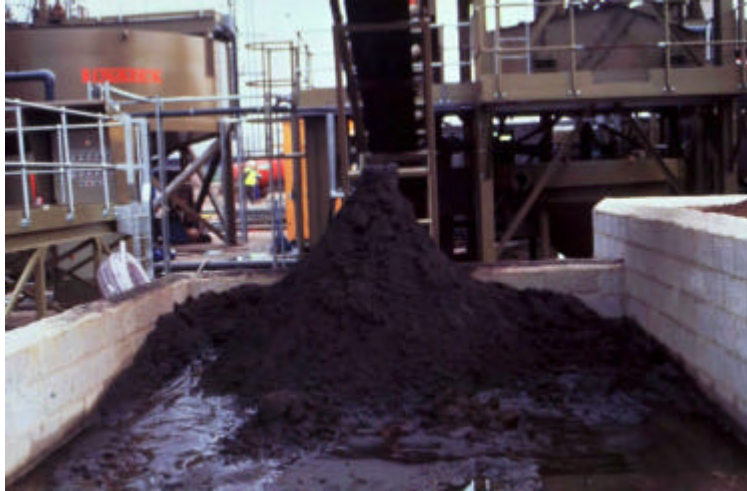
Plate 4: Contaminated stream from the dense medium separator, mostly consisting of contaminated peat and root fragments.
