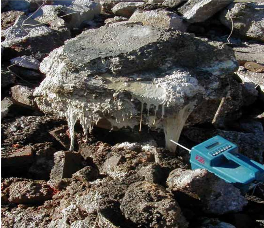
Plate 7.3: Use of PID to Measure VOC Concentration Following Exposure of Viscous White Product Containing Chlorinated Hydrocarbons.
