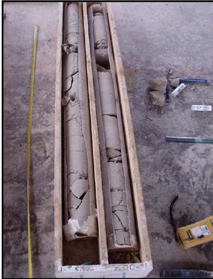
Plate 3.2: Fractured Grey Chalk from characterisation borehole
