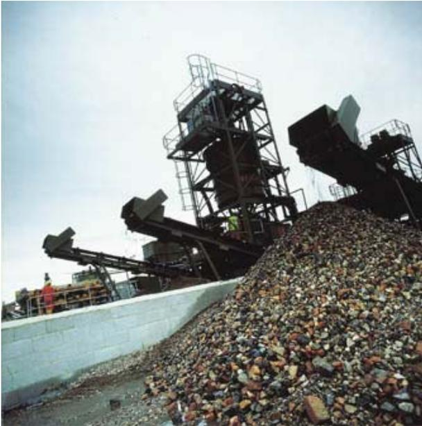
Clean coarse output from soil washing plant containing natural and made ground.
