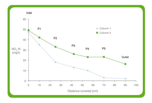
Figure 3.3: Results from the column experiments. Profile of nitrate concentrations (expressed as  $NO_3^--N$ ) along Columns 1 and 2. Different flow rates which equated to average residence times of 6.5 and 1.6 days for Column 1 and 2, respectively.
