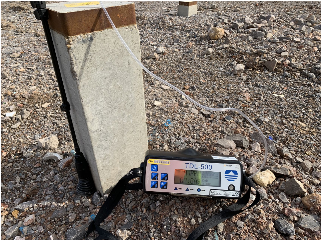
Figure A2.12: Monitoring for methane with tuneable diode laser
