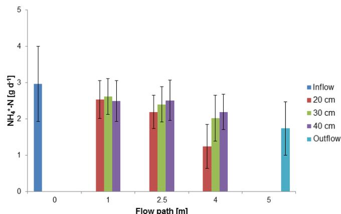
Figure 4: Average loads of  $\text{NH}_4^+\text{-N}$  in unplanted horizontal subsurface flow constructed wetland
