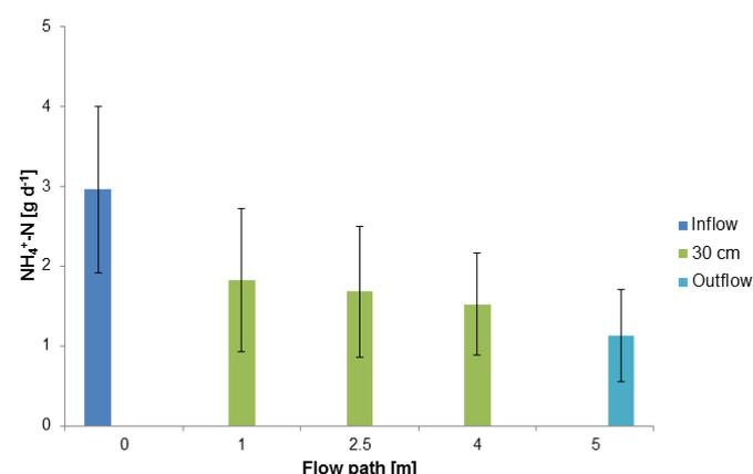
Figure 6: Average loads of  $\text{NH}_4^+\text{-N}$  in floating plant root mat
