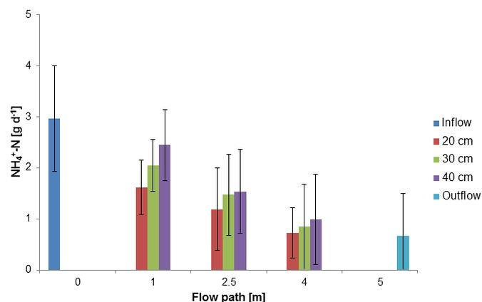
Figure 5: Average loads of  $\text{NH}_4^+\text{-N}$  in planted horizontal subsurface flow constructed wetland
