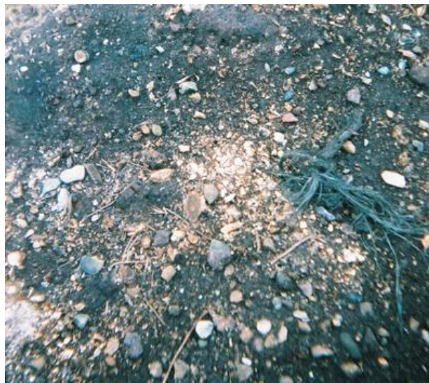
Photograph 62. Spent oxide in soils at a former gasworks. Source: Russell Thomas.
