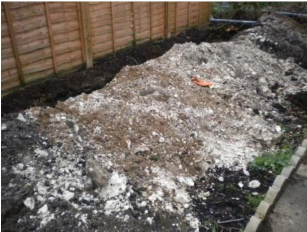
Photograph 36. Foul lime excavated on a former gasworks. Source: Parsons Brinckerhoff.
