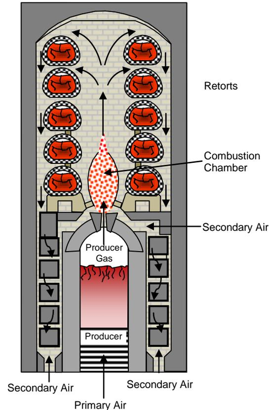
**Figure 6. Cross section of a horizontal retort, showing the gas producer. Based on historical drawings, Source: Russell Thomas.**
