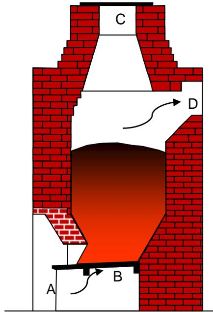
**Figure 1. Bischof Gas Producer.** Air was drawn into the producer (A) through the fire bars (B) and fuel, exiting via the vent (D). Fuel was loaded via door C. Source: Russell Thomas.
