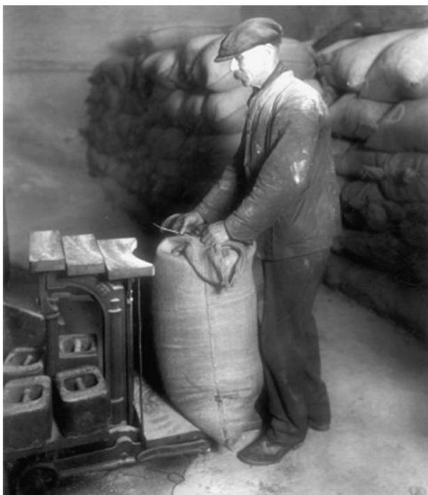
**Photograph 61. Bagging sulphate of ammonia fertiliser.**
