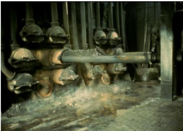
**Photograph 21. Loading a retort with a mechanical charger.**
