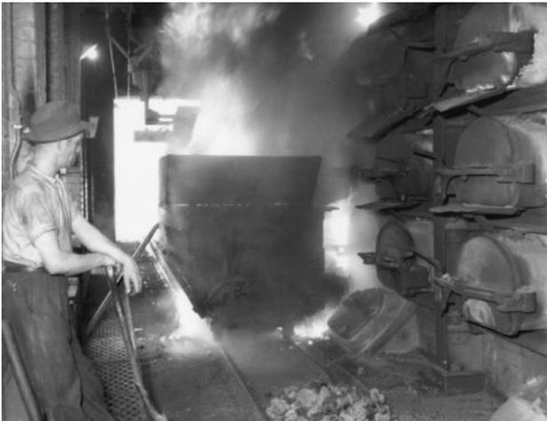
**Photograph 20. Unloading a through-ended retort mechanically.**
