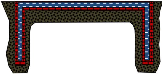
**Figure 14.** A schematic representation of an annular gasholder tank. Source: Russell Thomas.
