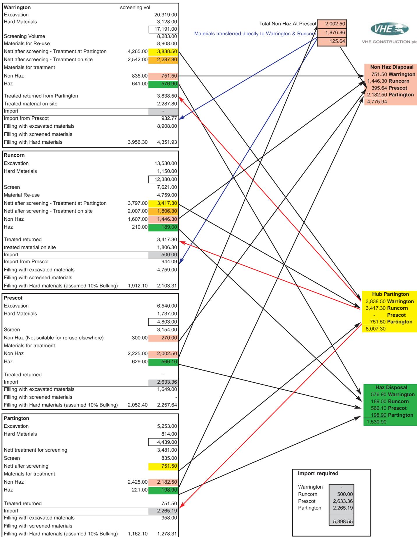
Figure 4: Tender stage Materials Management Plan (units are in m³)
