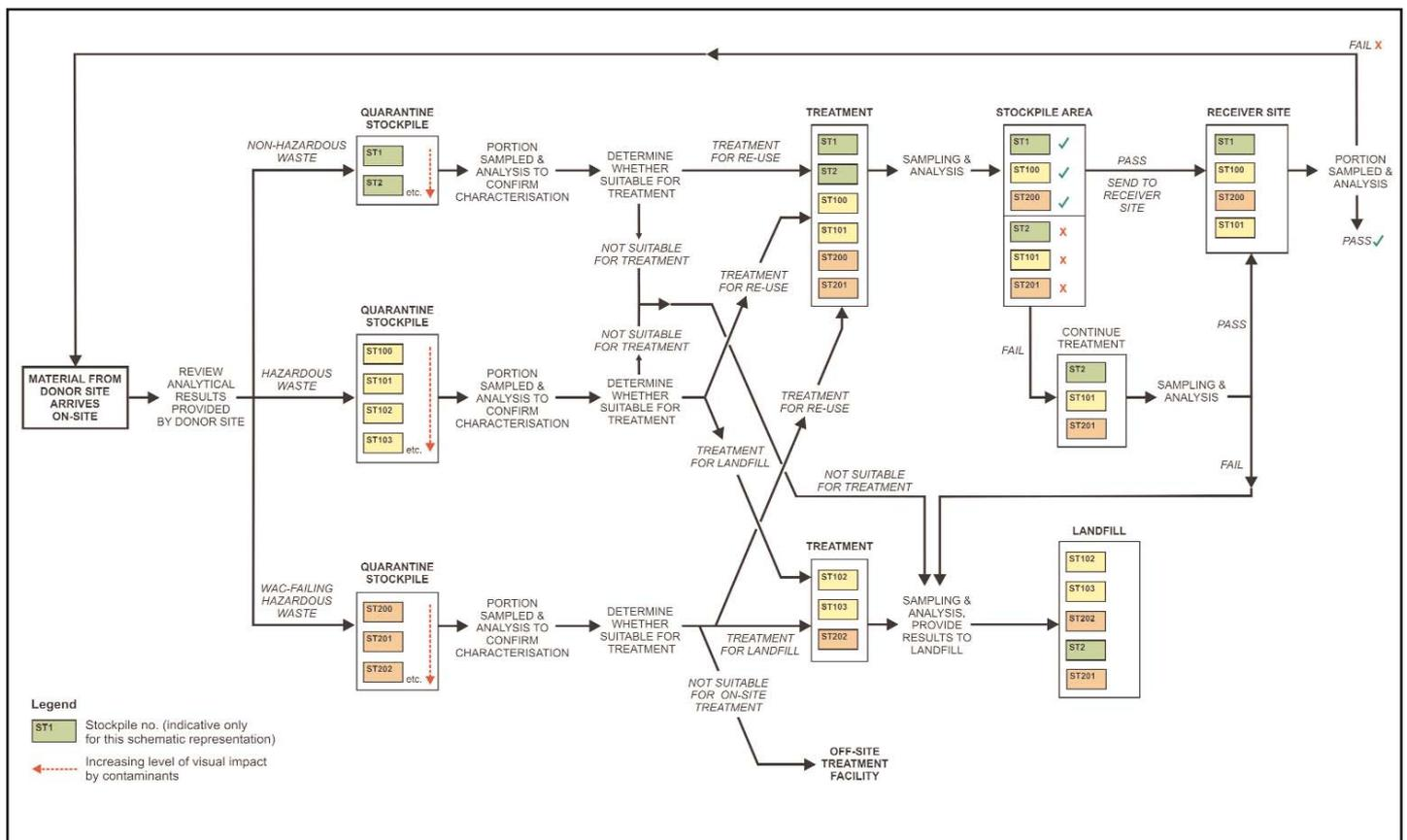
Figure 3: Schematic flowchart showing materials management.
