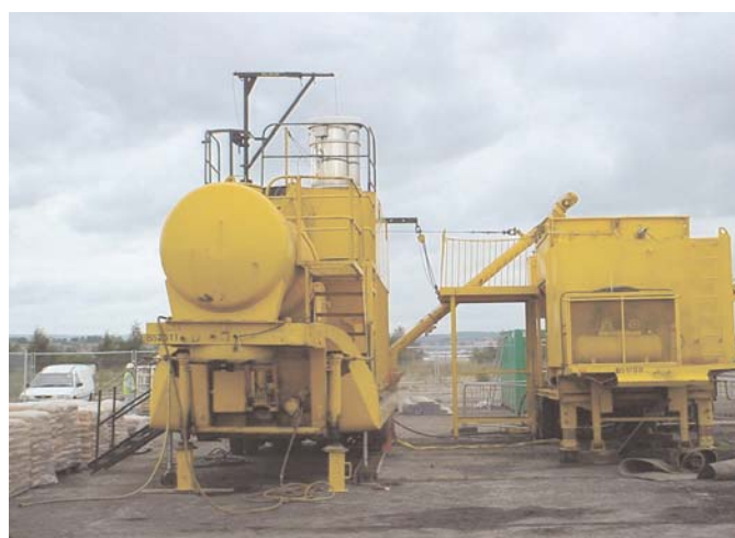
Figure 1: Site mixing equipment comprising silo (left) and Pugmill mixer (right).
