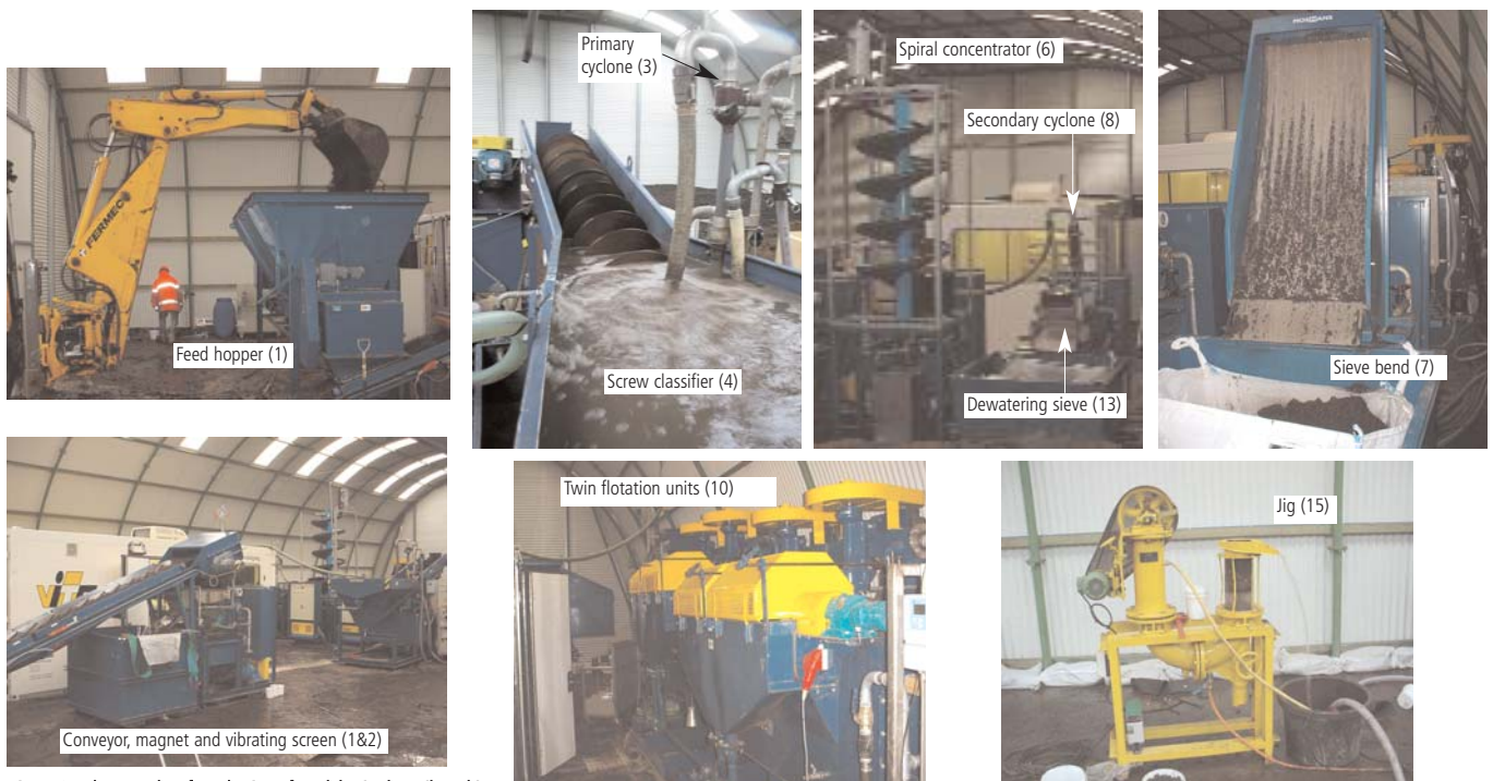
Figure 2. Photographs of a selection of modules in the soil washing process. The numbers correspond to the modules in Table 1.
