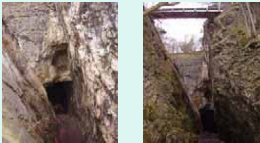
In this case the ore body forms a stable wedge
