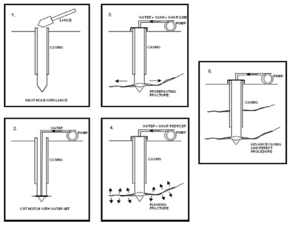
Figure 3 Hydrofracturing (after Schuring 2002)
