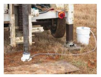
Figure 4.19: Pressurized air system for collecting dry samples and mitigating dust generation
