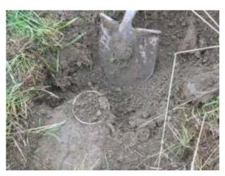
Figure 4.26: Hand extraction of a core sample at Astra Pyrotechnics site
