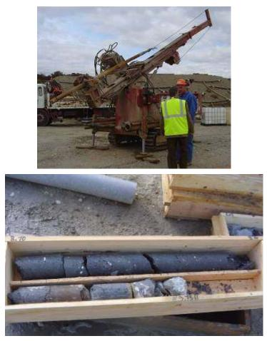
Figure 5.3: Image of the drilling machine used and an example of typical cores extracted
