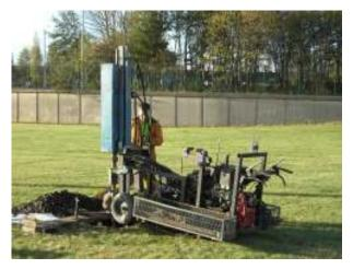
Figure 4.55: Equipment used for core extraction
