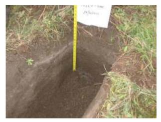
Figure 4.25: Trial pit at the Astra Pyrotechnics site, PC treated cell
